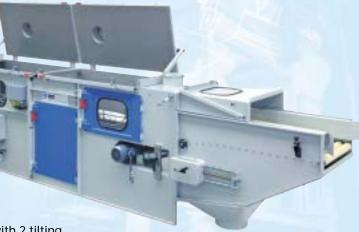
Complete bag slitting machine with cleaning unit, bag compactor and enclosed belt conveyor
